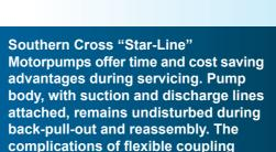
disassembly and realignment associated with long coupled pump units are also totally eliminated .
